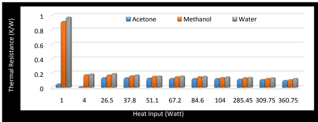
**Fig. 2** Thermal Resistance Of CLPHP With Acetone, Methanol And Water As Working Fluid
